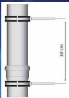
Figure 1. Pipe - pipe connection method
